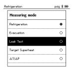
For the temperature-compensated leak test, a connection is established with available Bluetooth® probes. If cable probes are connected to the instrument, they are prioritized for the compensation. Please note that only air probes are ideal for temperaturecompensated leakage testing.
